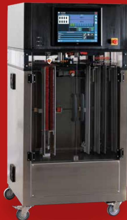
VisionScan Max is an objective, non-destructive alternative to the traditional blue dye leak test for blister packs with an automated feed magazine for minimal operator involvement. It enables pharmaceutical manufacturers and packagers to meet the stringent quality control requirements of the industry while reducing waste and costs. VisionScan Max generates accurate, reliable pass/fail results and its tool-less design improves efficiency where multiple product changeovers are required.
